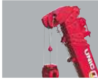
2 Automatic stop for overwinding
