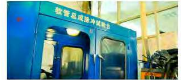
Millions Times of Life Tests on Rubber Hose
